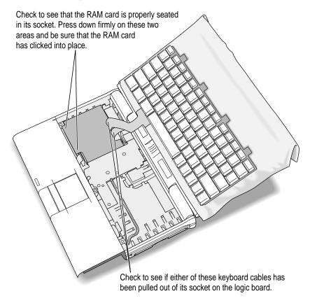
Make sure the keyboard cables are still properly connected.
